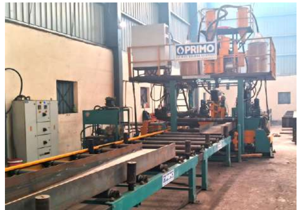
Automatic H-Beam Welding Line
